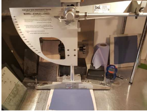
Image 1. Pendulum tester in-situ
